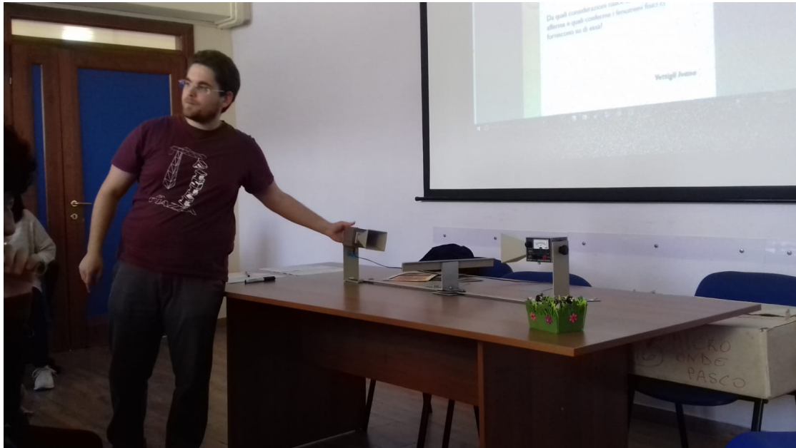
FIGURE 2.9: Myself at the Liceo Scientifico Carlo Urbani showing the functioning of the microwave apparatus. On the left is the radiating antenna, on the left the receiving antenna with a graduated scale to read the intensity of the current generated by the incoming radiation. In the middle, a support to add various material like polarizations plates, slit and double slits.
