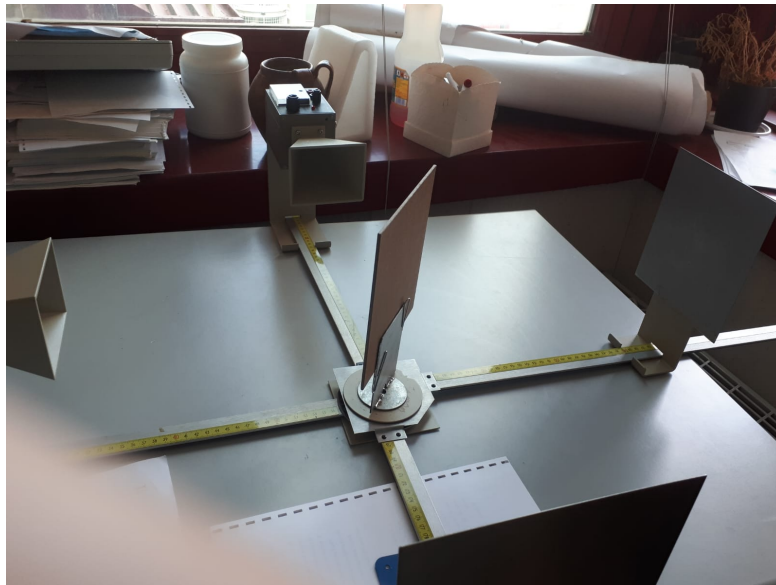
FIGURE 2.12: A Michelson interferometer with a microwave antenna a light source.
