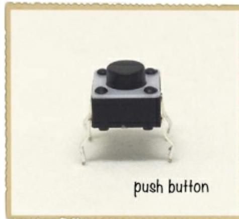
Plug the push button into your breadboard over the notch in the middle. Then, use a jumper wire to connect one side of the push button to the breadboard's positive supply column. Next, connect the positive wire from your battery clip to the other side of the push button. Finally, connect the negative battery clip wire to the negative supply column.
