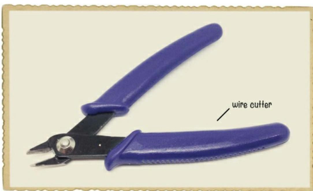
► A **wire cutter** (Jameco #35482, Bitsbox #TL008) to cut or remove the insulation from wire.
