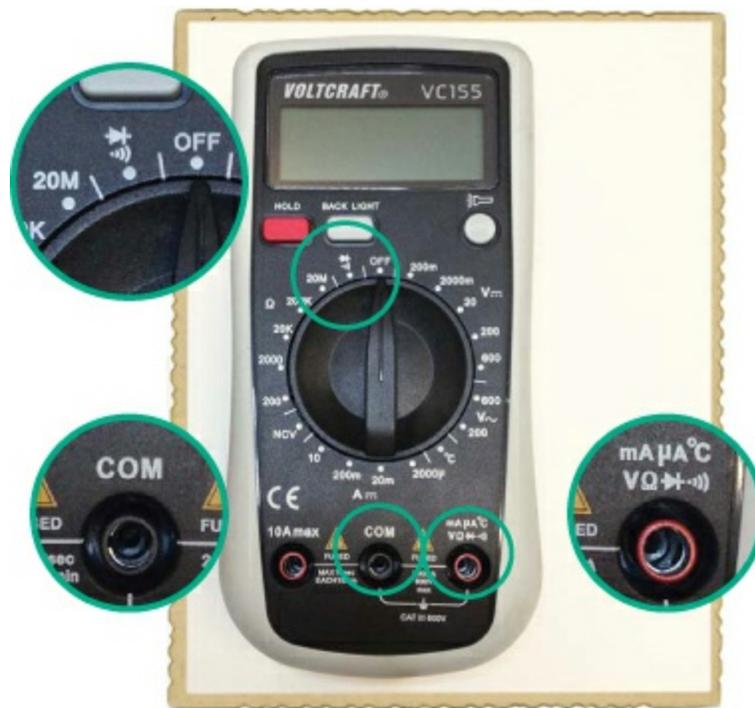
You don't want a direct connection between the positive and negative columns because that would short-circuit the battery and stop the game from working. Use the continuity tester to check for short circuits.
