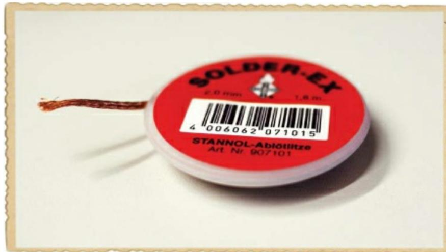
When you place a piece of solder wick on top of a solder joint and heat both together, the solder should melt as usual, and the solder wick should absorb the liquid solder just as a dry cloth absorbs water. When you remove the solder wick, the solder should be on the wick instead of on the circuit board!
