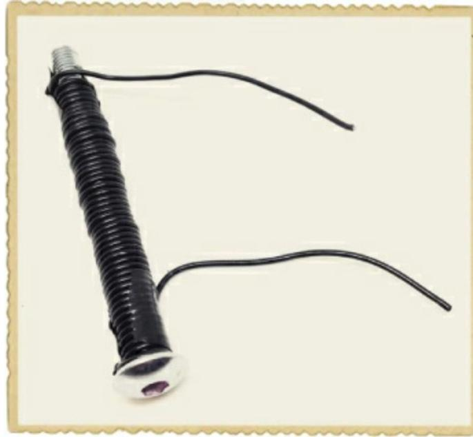
Wrap the wire as tight as possible and tape the end to make sure the turns stay in place. We call this wound wire the *coil* of the electromagnet.
