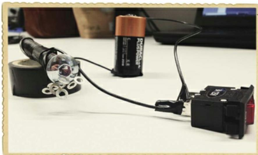
If nothing happens, press your switch into the other position; the bolt should start to pull the metal object now.
