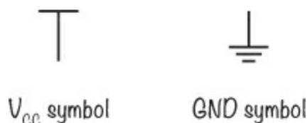
If nothing in the circuit diagram or its description says otherwise, you can assume that  $V_{CC}$  represents the positive side of the battery and that  $GND$  represents the negative side, or ground. The symbols sometimes look a little different, but the  $V_{CC}$  symbol usually shows a wire connecting down from its symbol to the circuit, while the  $GND$  symbol shows a wire connecting up from the symbol to the circuit.
