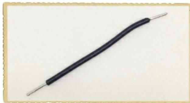
Cut a piece of wire about 2 inches long and strip about 0.3 inches of insulation from both ends. Removing insulation from shorter wires can be tricky, so if you're struggling with this step, use a longer wire instead. When you know what length of wire you can strip most easily, prepare two more wires. Then, solder the three wires to make the remaining connections.
