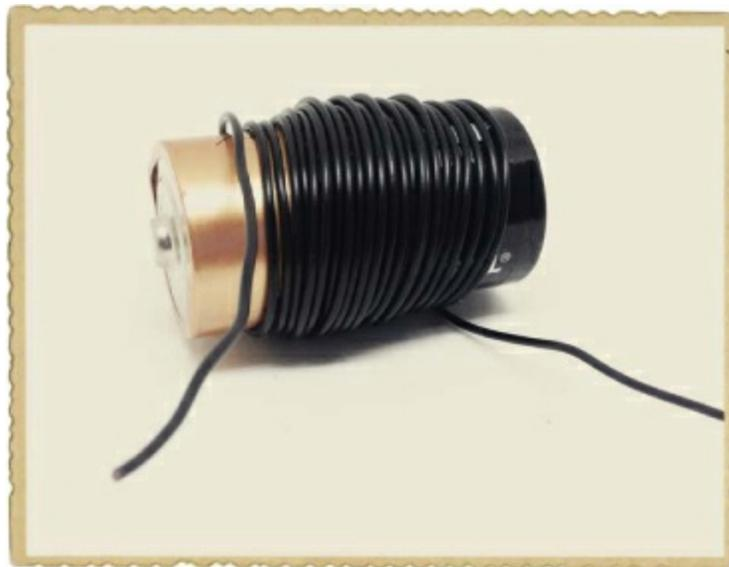
If you buy the wire I recommend in this project's Shopping List ([page 34](#)), try making around 30 windings; if you use thinner wire, wind it more. The point is to make the coil as magnetic as possible, without making it too heavy. More windings make the rotor more magnetic, but also heavier.
