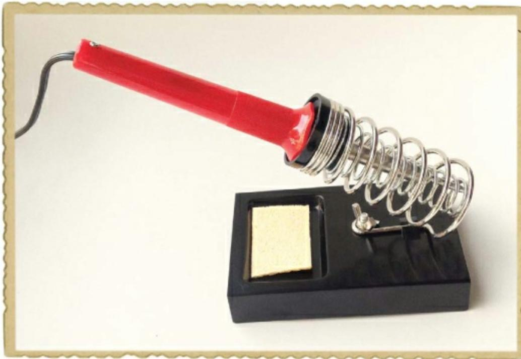
After a minute or two, check whether the iron is hot enough by touching some solder to the tip of the iron. If the solder melts, your iron is ready to go.
