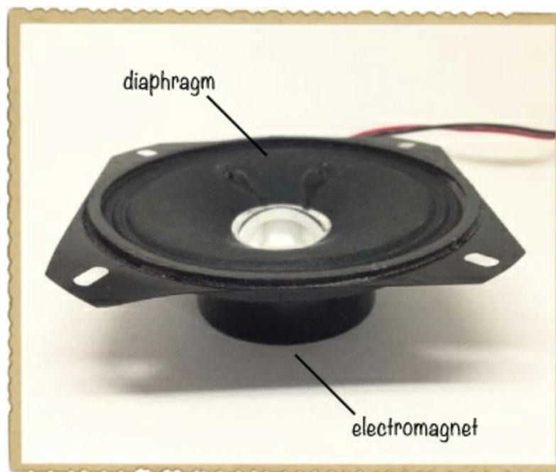
A loudspeaker has an electromagnet inside that moves a *diaphragm*, which is a surface that pushes the air in front of it. If a circuit turns the power to the loudspeaker's electromagnet on and off at, say, 1,000 times per second, then the diaphragm pushes the air back and forth 1,000 times per second. This is called the *frequency* of the sound, and frequency is measured in hertz (Hz). A frequency of 1,000 times per second, or 1,000 Hz, creates a steady beep.
