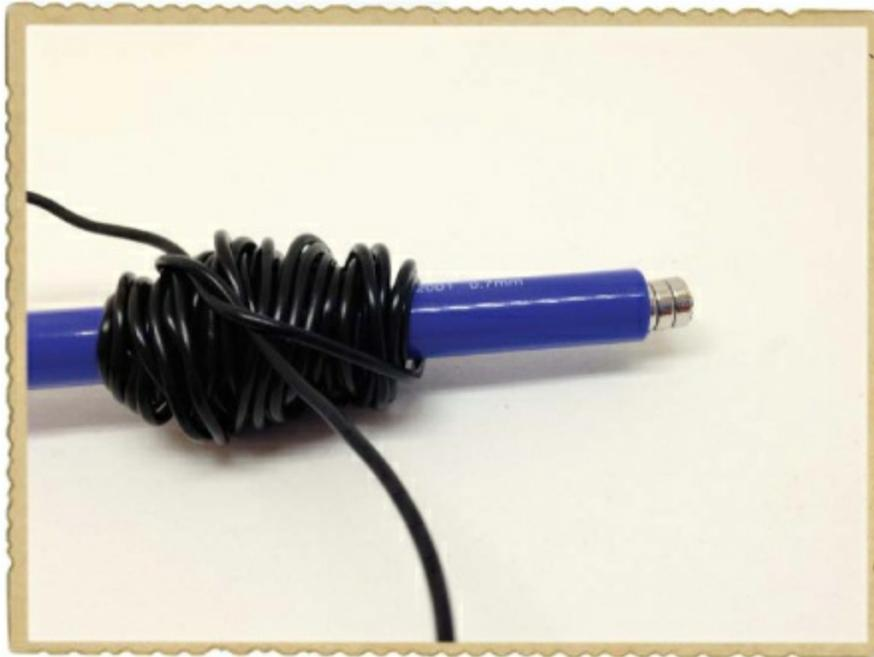
Holding the tube and multimeter leads in your hand, place one finger on each side of the tube so that the magnets don't fall out. Then, shake it like you mean it!
