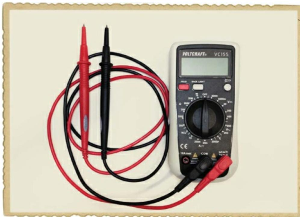
The red lead is the positive lead, the black lead is the negative lead, and the big dial in the middle lets you tell the multimeter what to measure. If you're having problems with a circuit, measuring the voltage at key points in your circuit is one practical way to figure out what's wrong.
